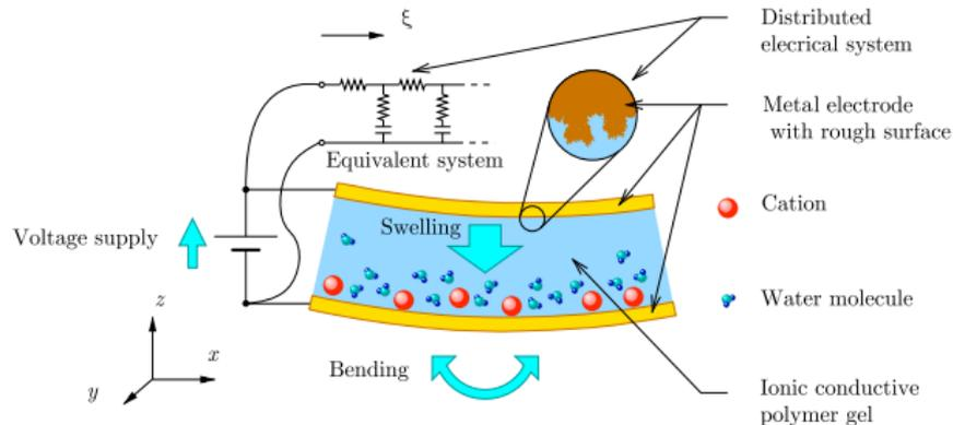
Fig. 2. Physical structure of IPMC.
