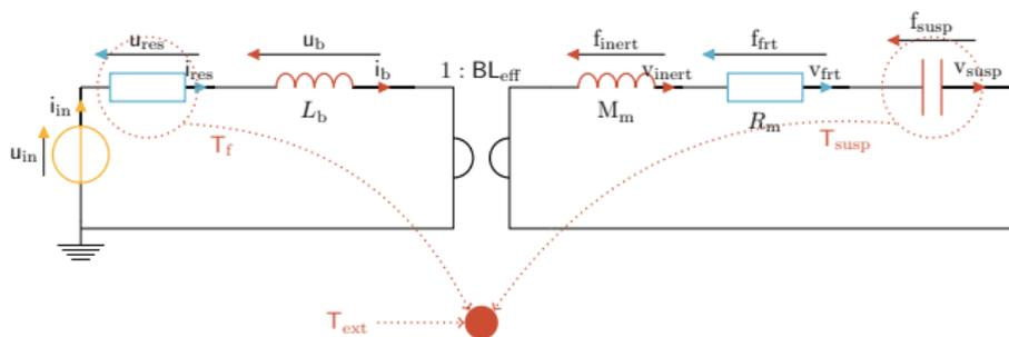
Figure: *Model of loudspeaker [T. Lebrun, Thèse doctorat , IRCAM, Paris, 2019]*
